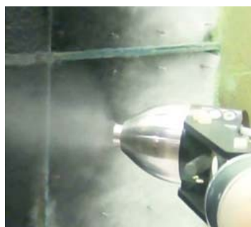
Industrial Bell/ Solvent Material Application
